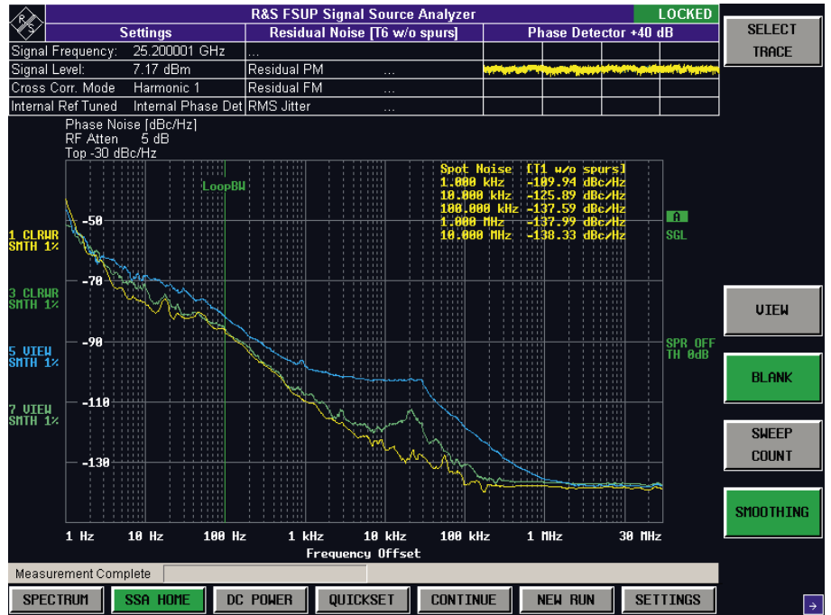
FIG 1 Phase noise measurement on a quality signal source at an input frequency of 25.2 GHz: without cross-correlation (blue), with approx. 1000 averages (green), and with approx. 20000 averages (yellow).
